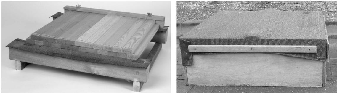
**Figure 7.4-1. Left: Photograph showing the double-layer set-up with the upper layer shifted 25 mm horizontally to the lower layer. Specimens are separated with bitumen foil from CCB-impregnated support beams. Right: Artificial shading by textile sheet of double layer test set.**
