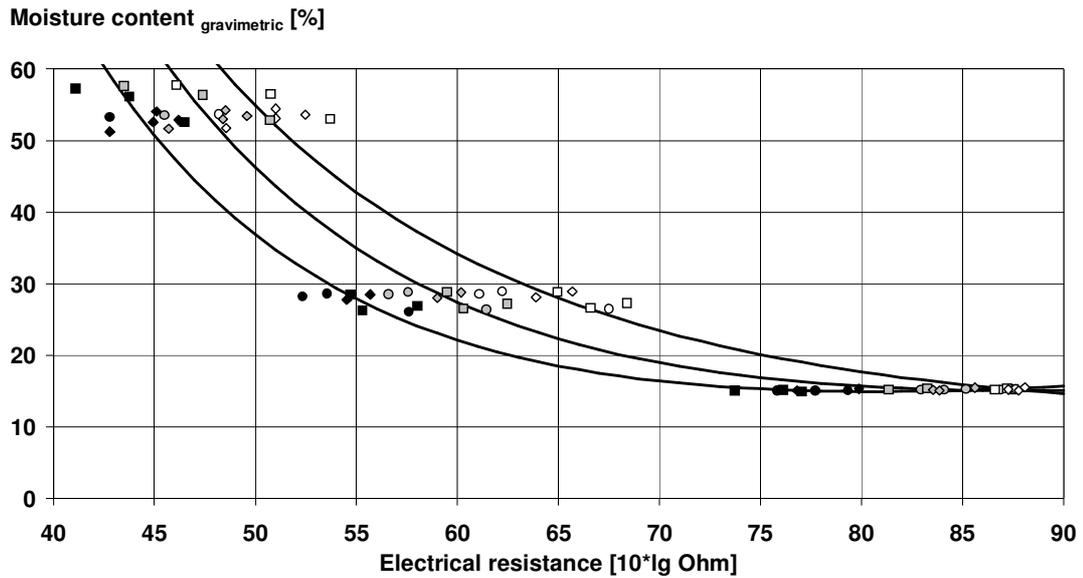
Figure 7.2-5. Resistance characteristic for Scots pine sapwood (○ = provenance 1, □ = provenance 2, ◇ = provenance 3, black filled marks = 36°C, grey filled marks = 20°C, non-filled marks = 4°C).
