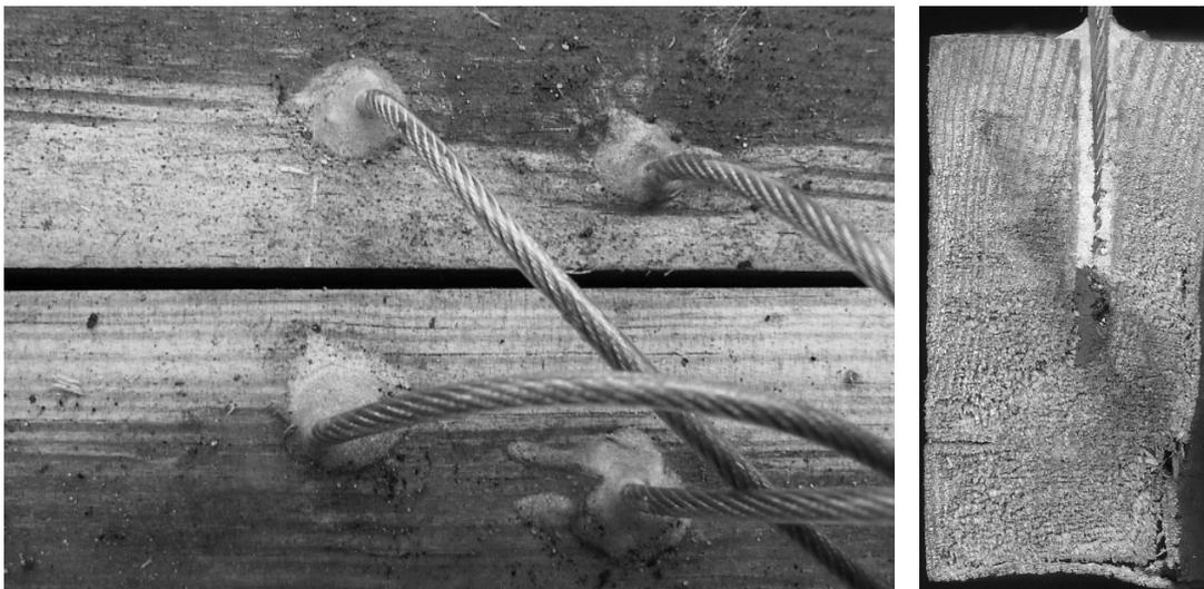
**Figure 7.2-9. Glued electrodes in Scots pine specimens. Left: After six years in the field. Right: Cross cut through a glued electrode in wood decayed by severe white rot after four years of exposure.**
