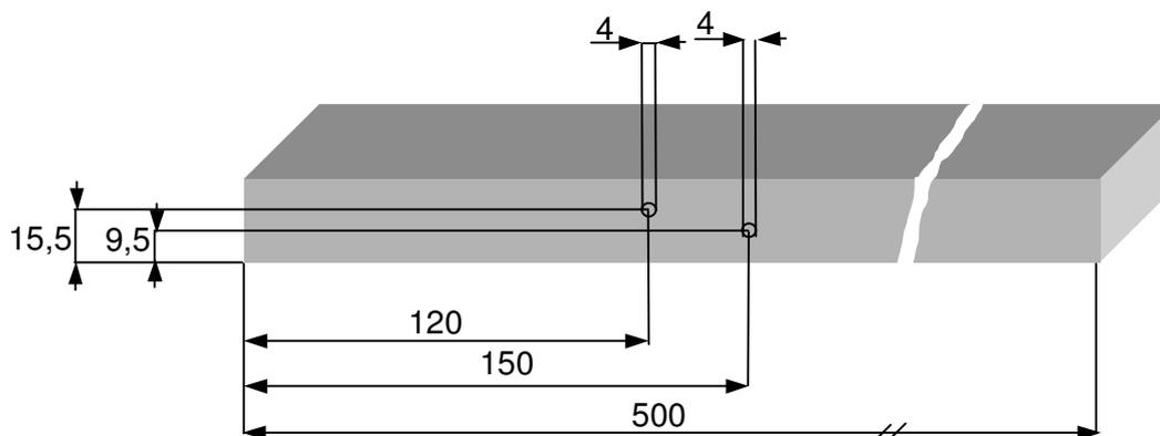
**Figure 7.2-1. Specimen according to EN 252 [11] and position of holes for installation of electrodes (all dimensions in mm).**
