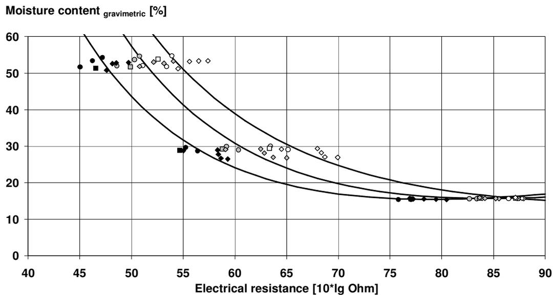
Figure 7.2-4. Resistance characteristic for spruce (○ = provenance 1, □ = provenance 2, ◇ = provenance 3, black filled marks = 36°C, grey filled marks = 20°C, non-filled marks = 4°C).
