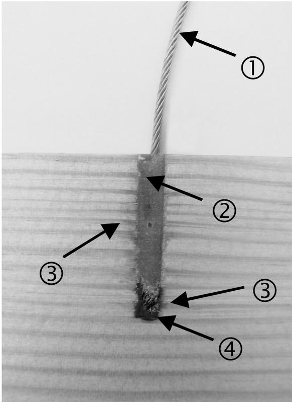
**Figure 7.2-3. Cross cut through a glued electrode. The polyamide coated stainless steel cable ① is glued in predrilled holes. On the bottom of the hole the uncoated cable is glued with the conductive glue ④, the upper part of the coated cable is glued with the isolating glue ②. The glue has penetrated into the lumina of the tracheids and produces a very durable connection ③.**
