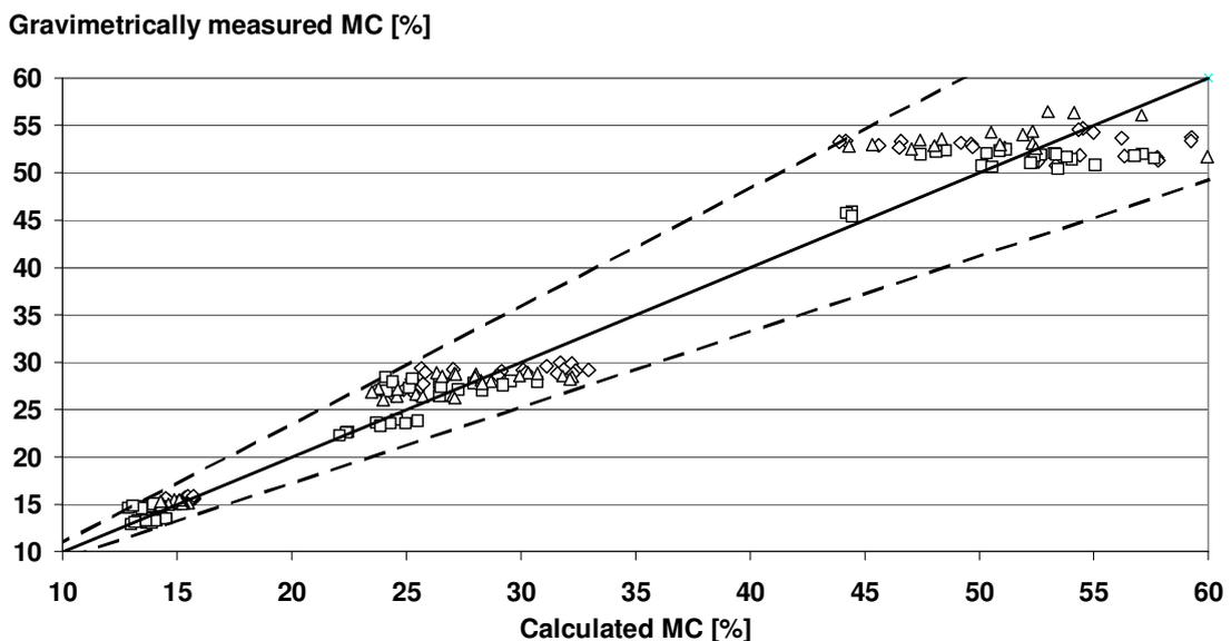
**Figure 7.2-7. Calculated MC compared with gravimetrically measured MC. Underlying regressions were determined for all provenances pooled together ( $\Delta$  = Scots pine sap,  $\square$  = Douglas fir,  $\diamond$  = Norway spruce).**
