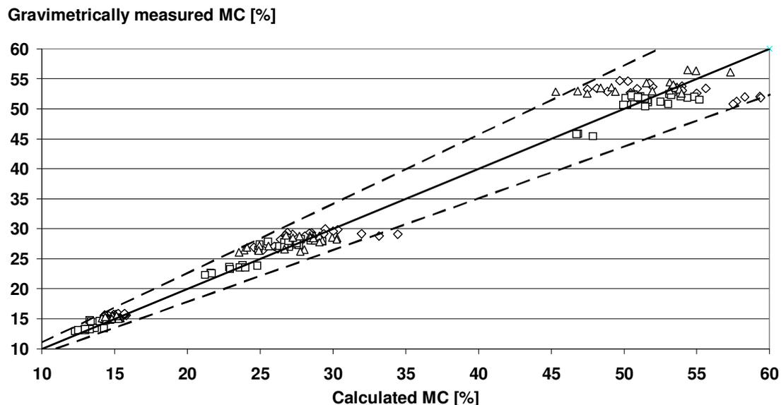
Figure 7.2-8. Calculated MC compared with gravimetrically measured MC. Underlying regressions were determined separately for the different provenances ( $\Delta$  = Scots pine sap,  $\square$  = Douglas fir,  $\diamond$  = Norway spruce).
