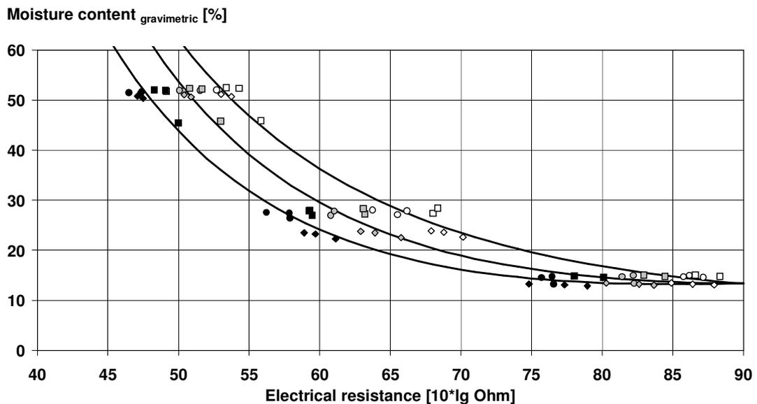
Figure 7.2-6. Resistance characteristic for Douglas fir (○ = provenance 1, □ = provenance 2, ◇ = provenance 3, black filled marks = 36°C, grey filled marks = 20°C, non-filled marks = 4°C).
