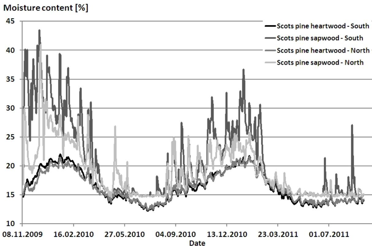
Figure 8: Wood moisture content of Scots pine sapwood and Scots pine heartwood on the North and South oriented facade from 09. 11. 2009 to 05. 09. 2011
