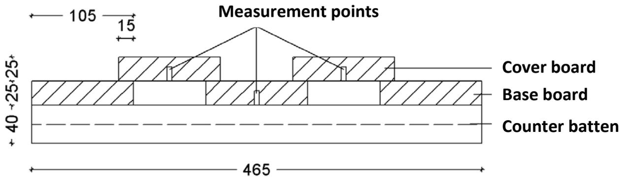
Figure 4: Position of measurement points in the board-on-board cladding of the test house (dimensions in mm)
