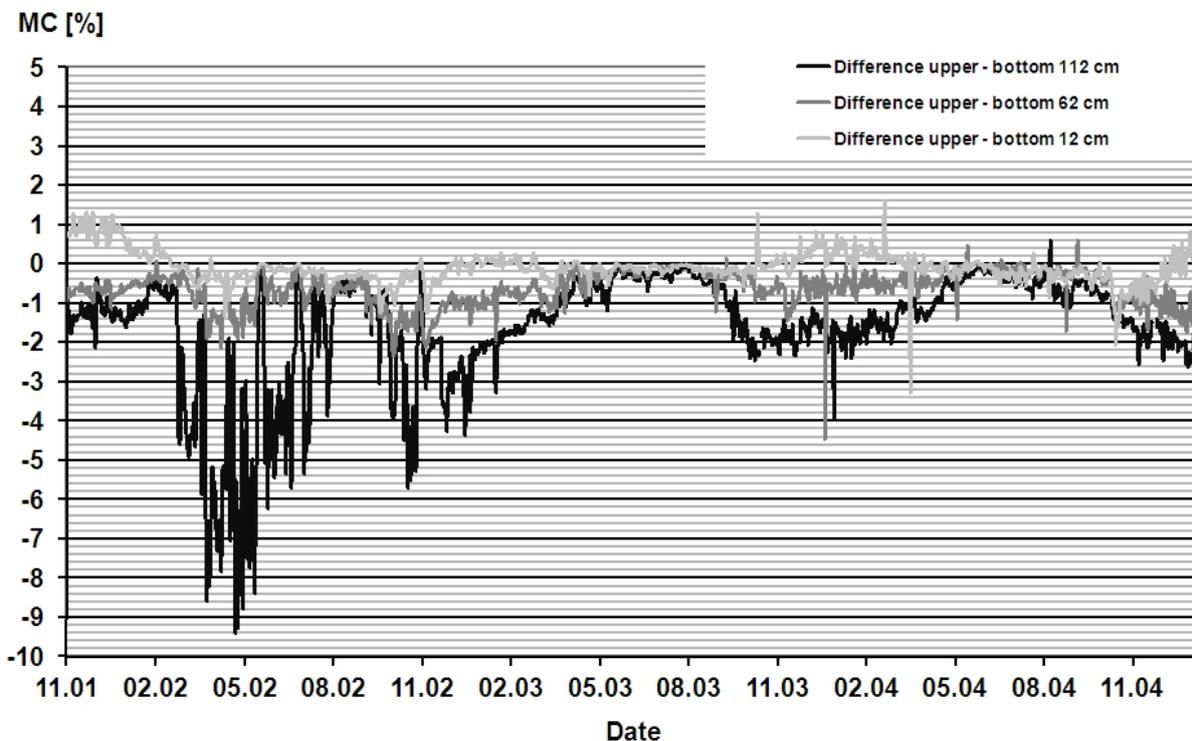
Figure 9: Difference of wood moisture content of upper and bottom wall for Norway spruce for all roof overhangs from 23.11.2001 to 10.01.2005
