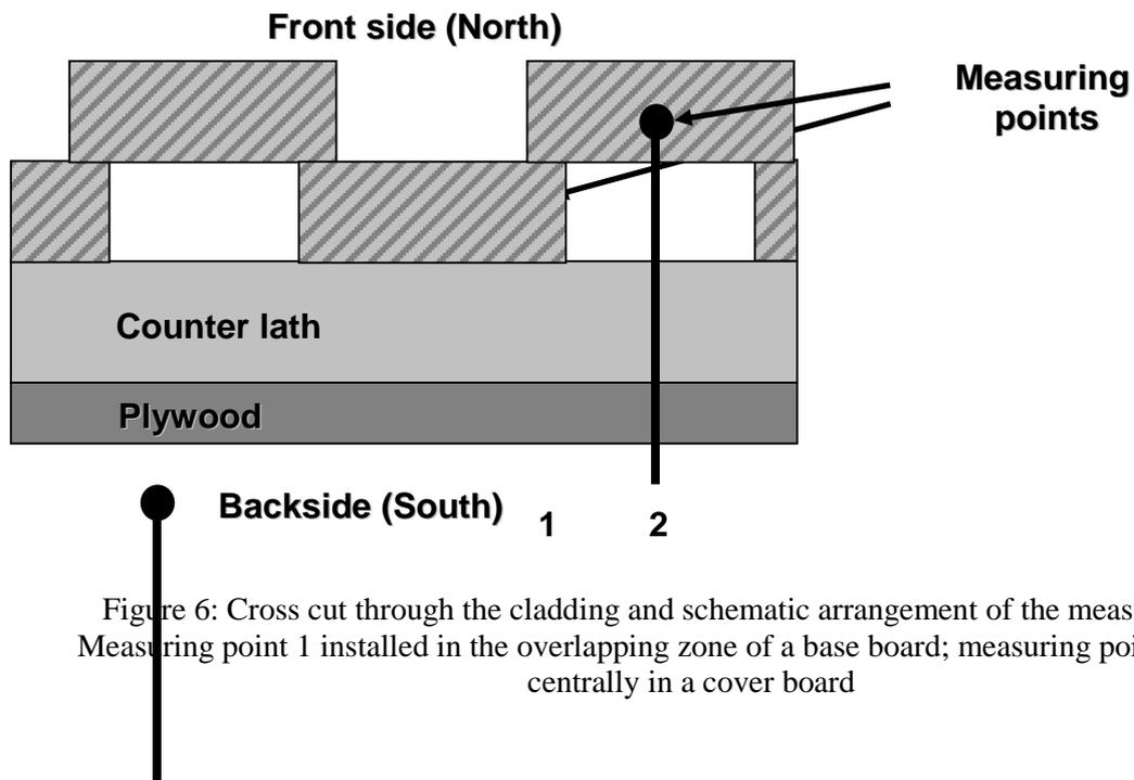
Figure 6: Cross cut through the cladding and schematic arrangement of the measurement points. Measuring point 1 installed in the overlapping zone of a base board; measuring point 2 installed centrally in a cover board
