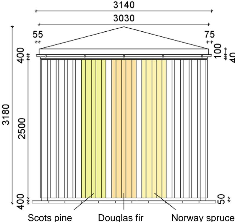
Figure 3: Position of test boards from different wood species in the board-on-board cladding of the test house (dimensions in mm)
