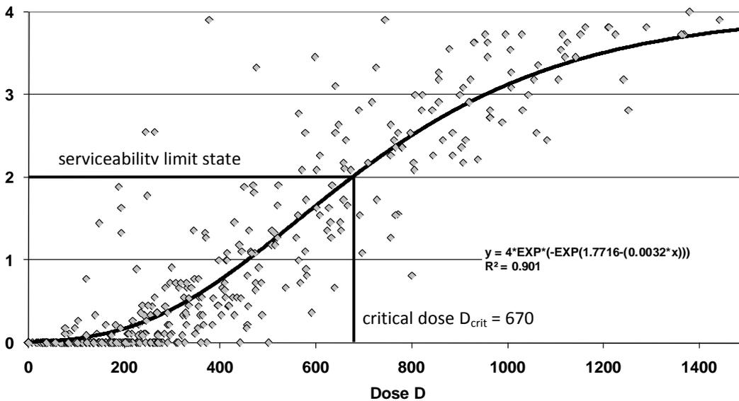
Figure 7: Relationship between the dose D and the mean decay rating according to EN 252 (1989) of Scots pine sapwood and Douglas fir heartwood specimens exposed at 23 different field test sites (each dot represents the mean decay rating for one wood species at one exposure site at a certain time of exposure; black line: Gompertz smoothing function), from: Brischke and Rapp 2010
