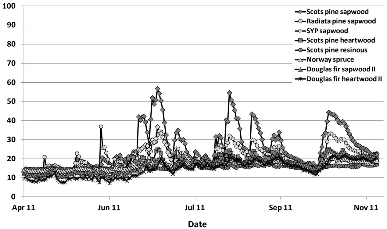
Figure 15: Moisture course of native softwoods exposed in sandwich tests in Hannover
