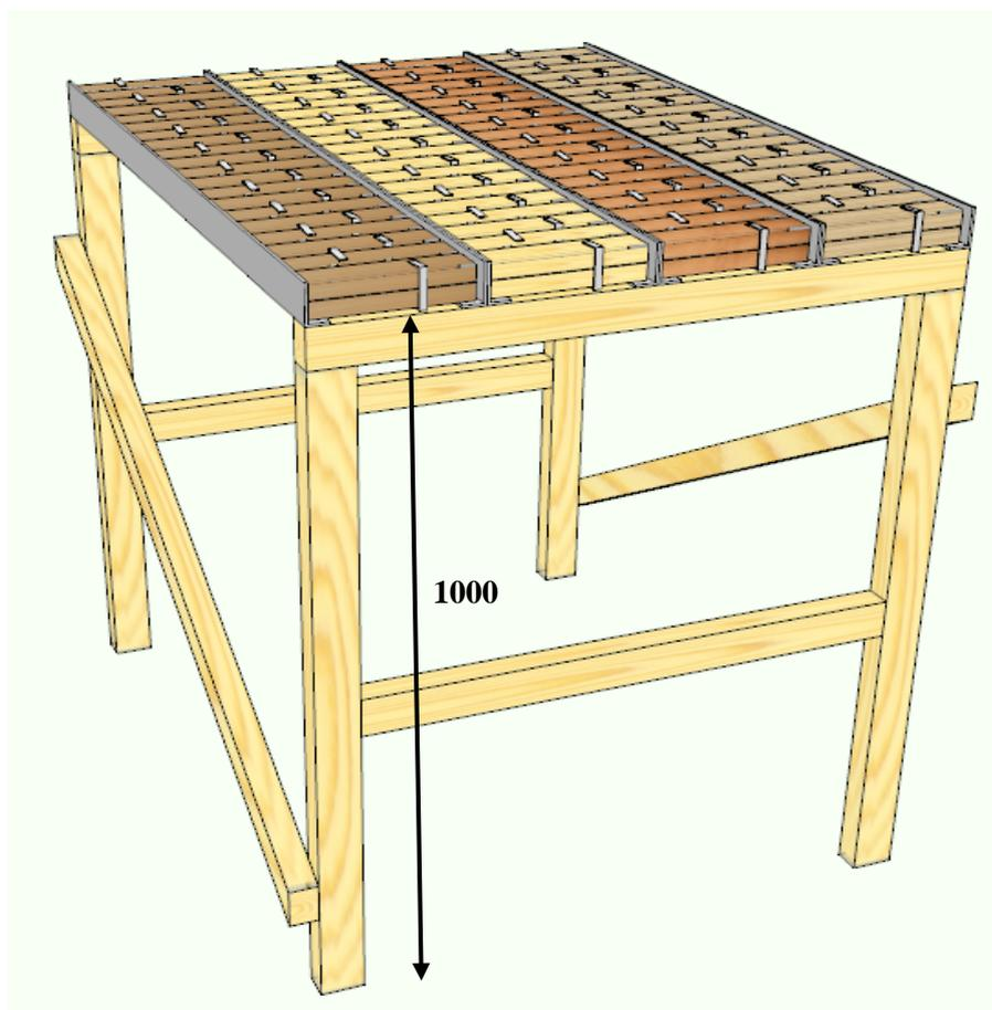
Figure 6: Sandwich test rig in Hannover, all dimensions in millimeter
