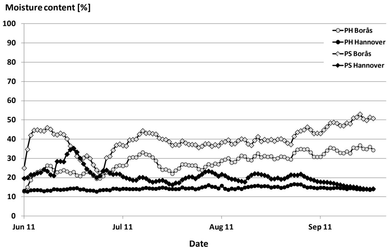
Figure 22: Moisture course of Scots pine heartwood (PH) and Scots pine sapwood (PS) exposed in Borås and Hannover in double layer tests
