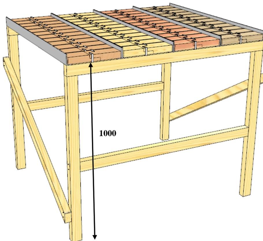
Figure 4: Lap joint test rig in Hannover and Borås, all dimensions in millimeter
