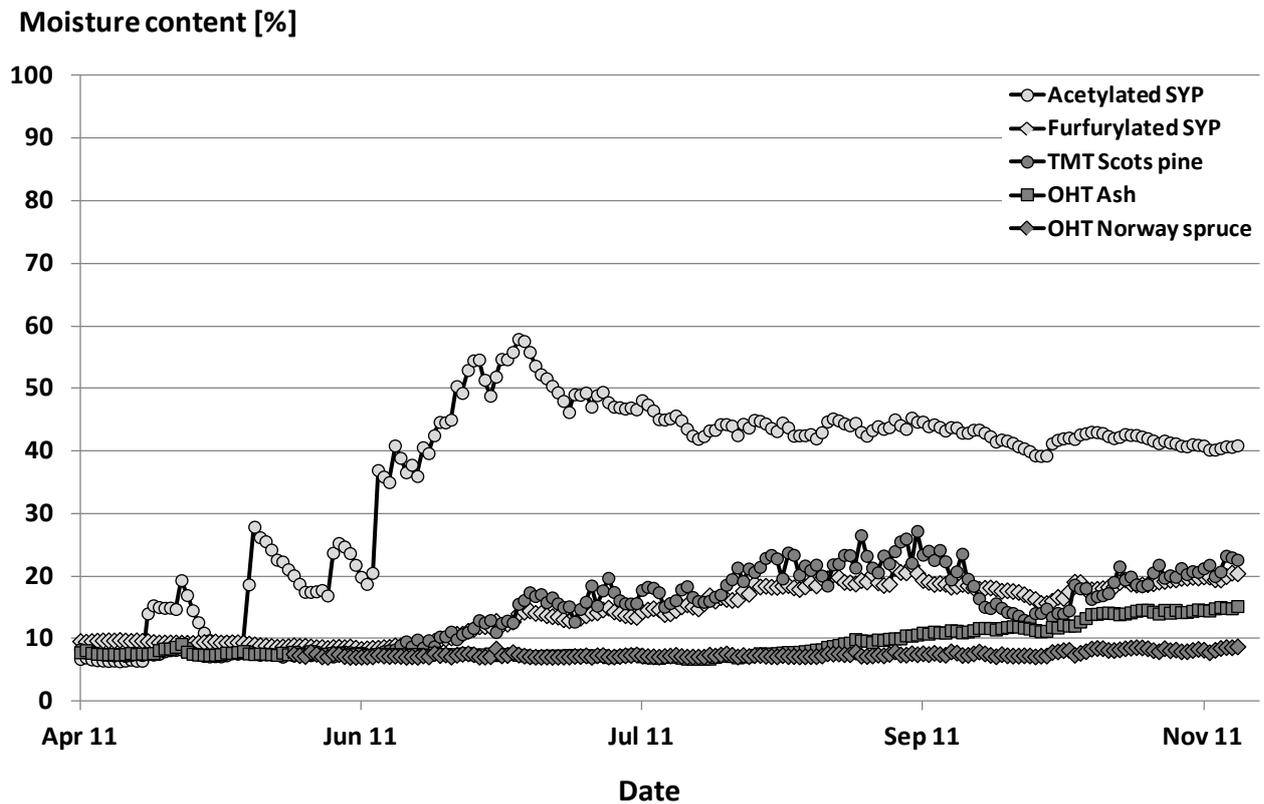
Figure 16: Moisture course of modified timber exposed in double layer tests in Hannover
