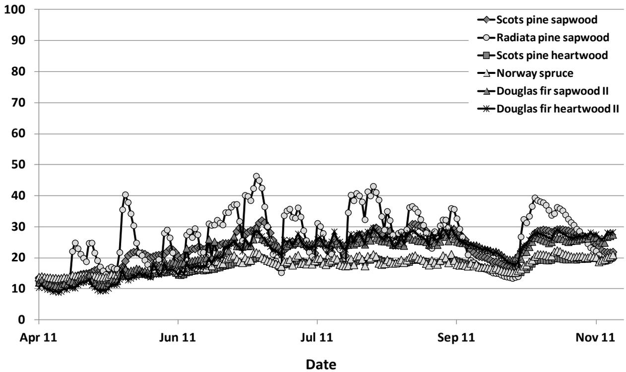
Figure 14: Moisture course of native softwoods exposed in lap joint tests in Hannover
