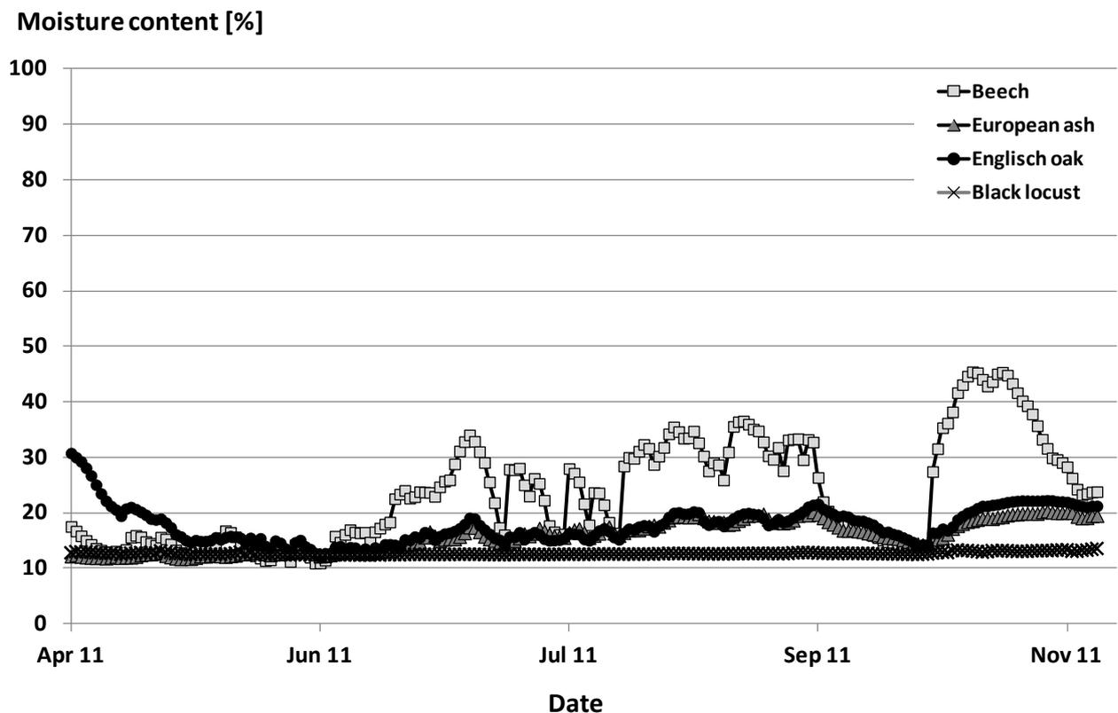
Figure 10: Moisture course of native hardwoods exposed in double layer tests in Hannover
