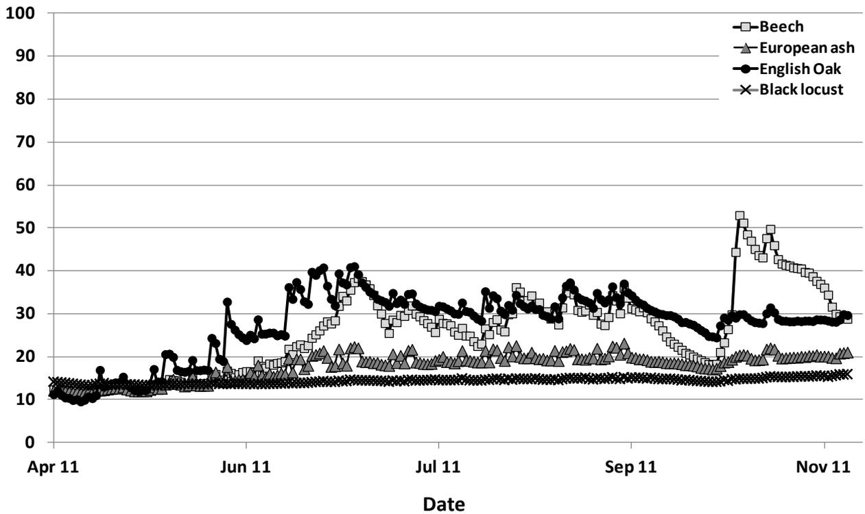
Figure 11: Moisture course of native hardwoods exposed in lap joint tests in Hannover
