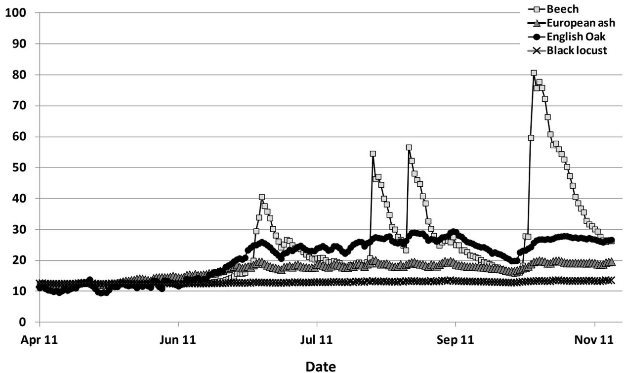
Figure 12: Moisture course of native hardwoods exposed in sandwich tests in Hannover
