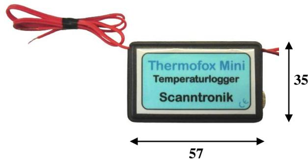
Figure 8: Data logging device ,Thermofox Mini‘, all dimensions in millimeter
