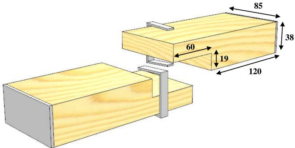
Figure 3: Exploded view of lap joint specimen, all dimensions in millimeter
