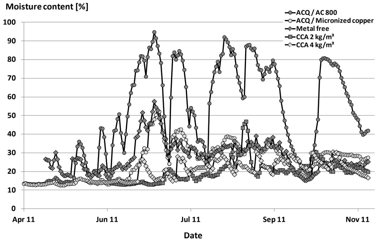
Figure 19: Moisture course of preservative treated timber exposed in double layer tests in Hannover
