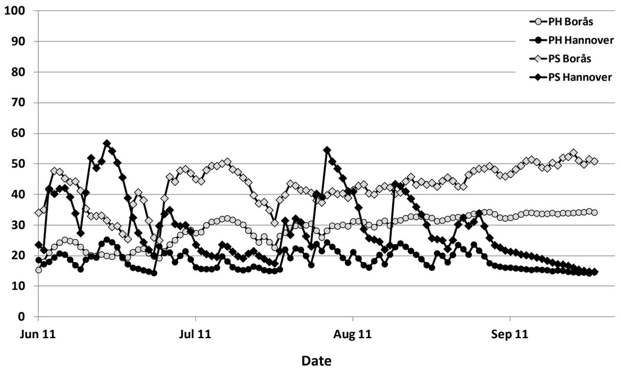
Figure 24: Moisture course of Scots pine heartwood (PH) and Scots pine sapwood (PS) exposed in Borås and Hannover in sandwich tests
