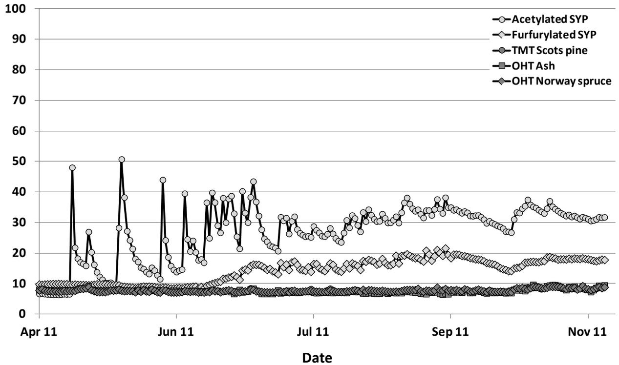
Figure 18: Moisture course of modified timber exposed in sandwich tests in Hannover
