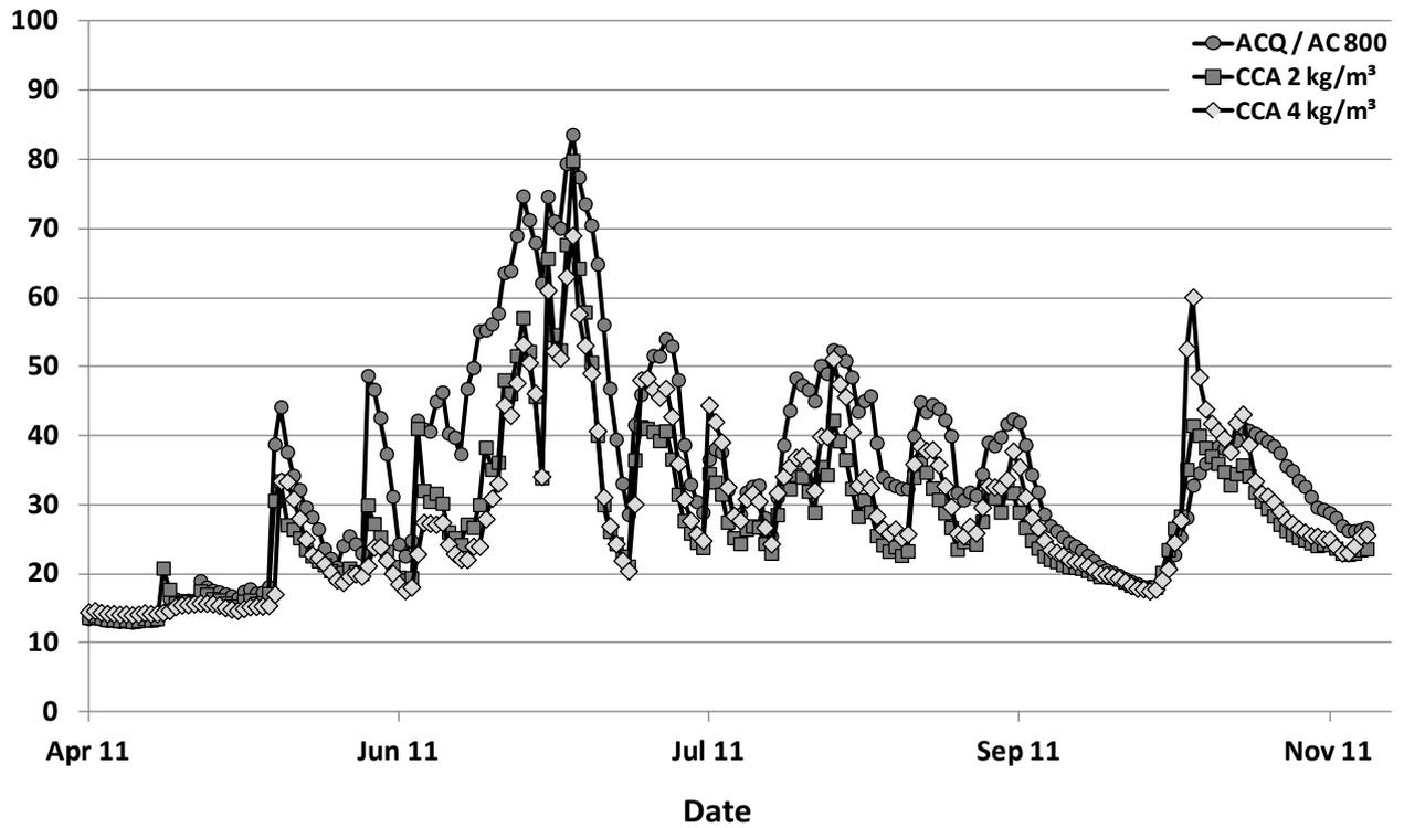
Figure 20: Moisture course of preservative treated timber exposed in lap joint tests in Hannover
