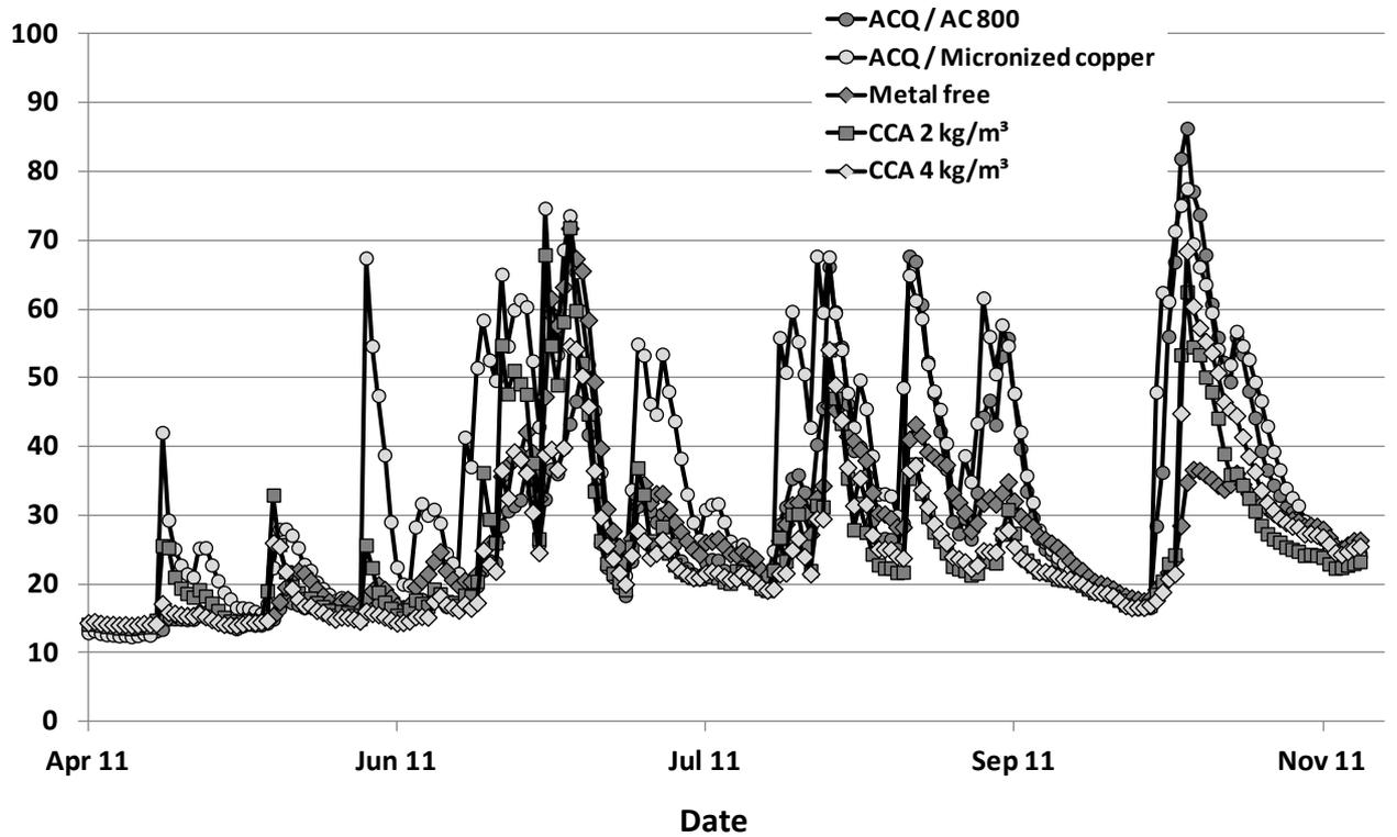
Figure 21: Moisture course of preservative treated timber exposed in sandwich tests in Hannover
