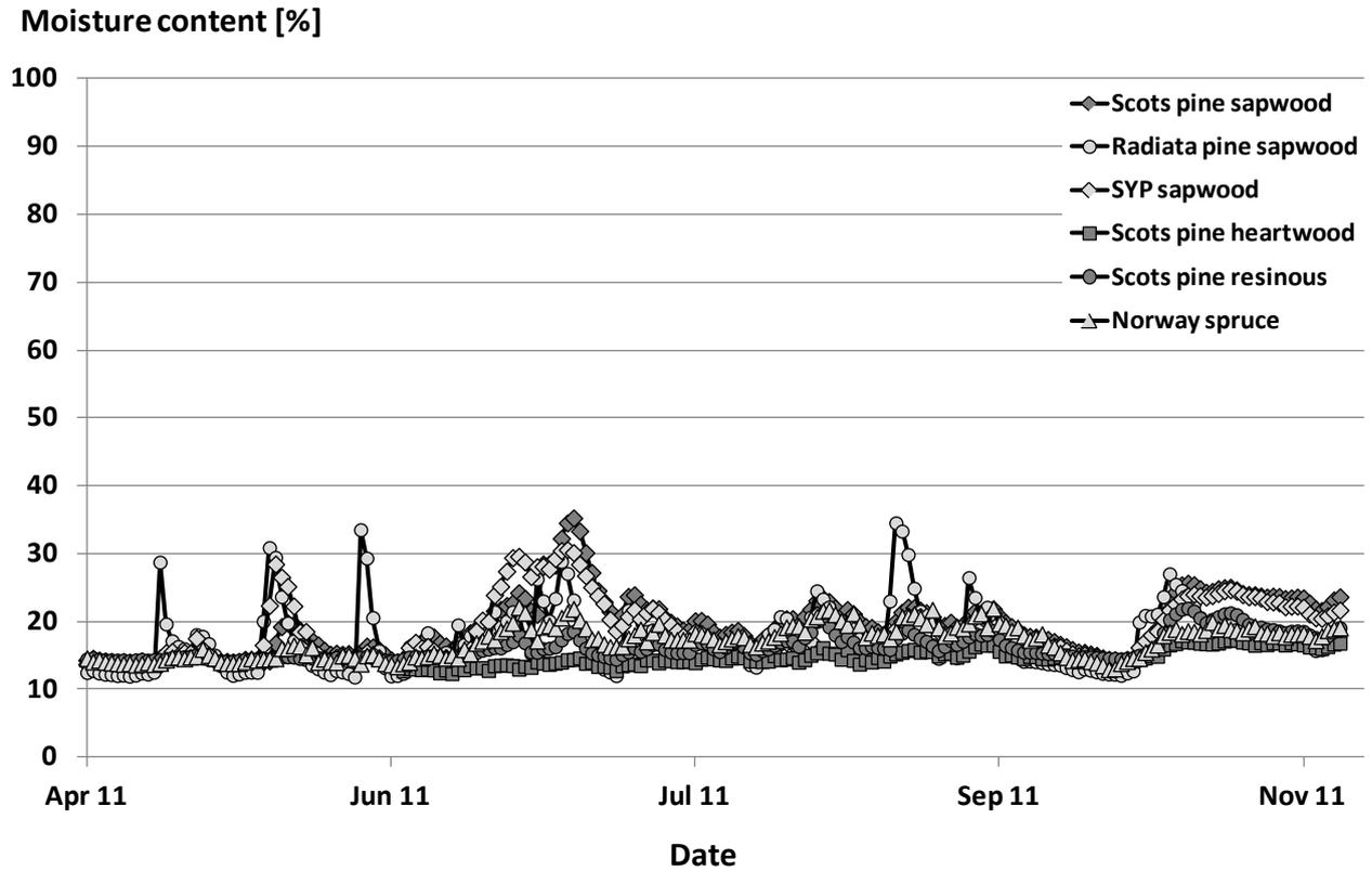
Figure 13: Moisture course of native softwoods exposed in double layer tests in Hannover
