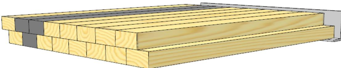
Figure 2: Double layer test (PE spacers in black)
