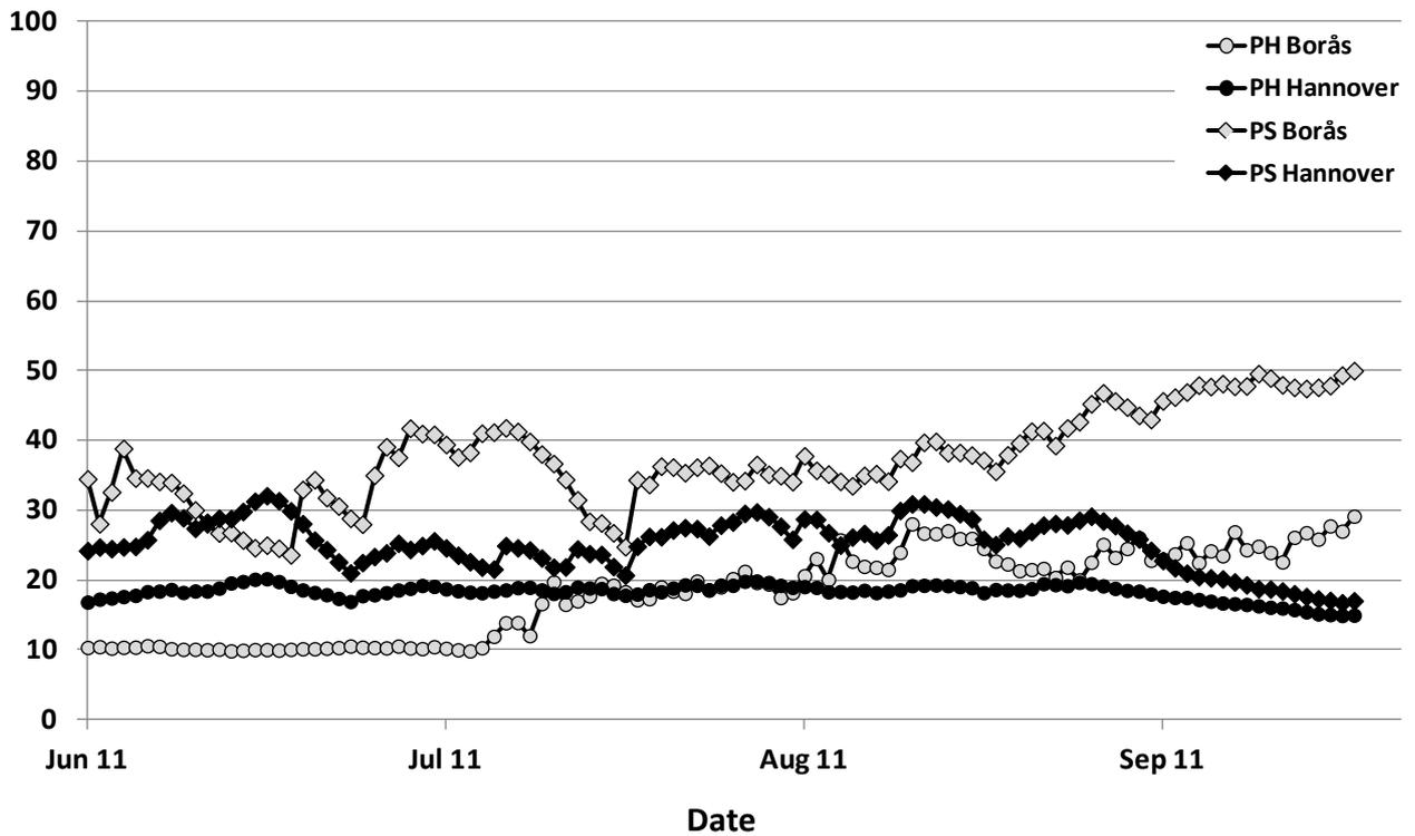
Figure 23: Moisture course of Scots pine heartwood (PH) and Scots pine sapwood (PS) exposed in Borås and Hannover in lap joint tests
