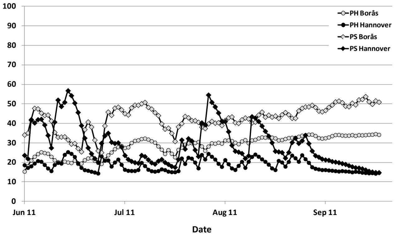
Figure 24: Moisture course of Scots pine heartwood (PH) and Scots pine sapwood (PS) exposed in Borås and Hannover in sandwich tests
