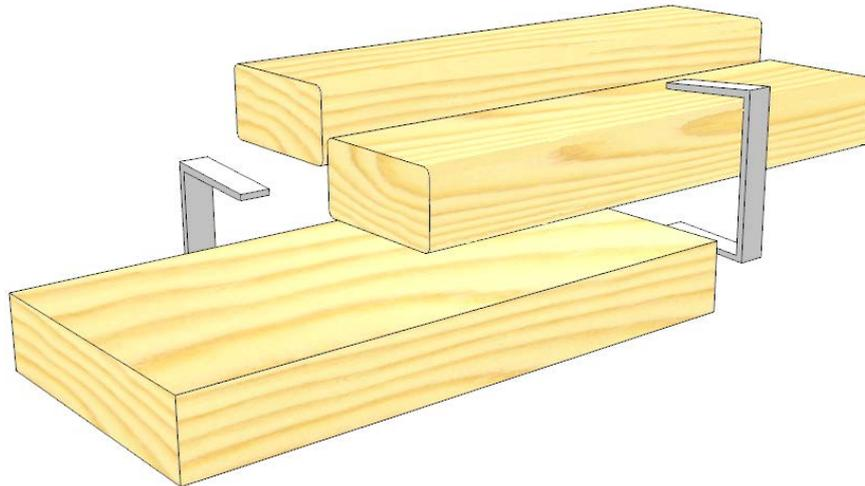
Figure 5: Exploded view of sandwich specimen
