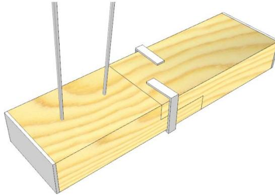
Figure 9: Lap joint specimen (upside down) with electrodes installed at the bottom side
