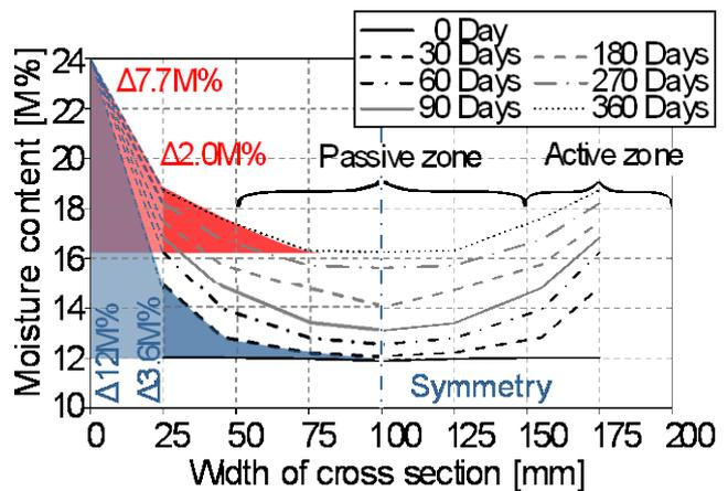
Figure 12: Experimental results of moisture distribution in tangential direction for the adsorption process, 200/200/200 mm
