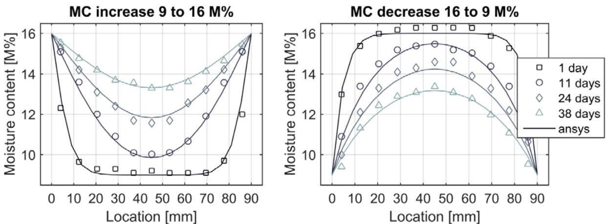
Figure 7: Comparison of experiments and simulations of wetting and drying process of a 90 mm wide beam
