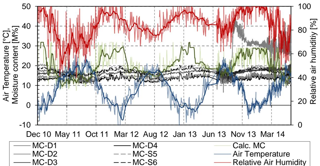
Figure 6: Timber bridge Obermatt, Measured climate and moisture content and calculated equilibrium moisture content
