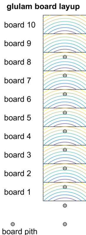
Figure 17: Glulam beam 100/400 mm with pith location on centerline and 50 mm under board edge
