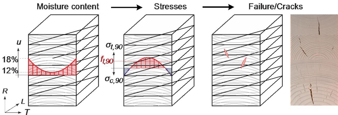
Figure 1: Moisture and stress distribution as well as failure of the cross section for an adsorption process
