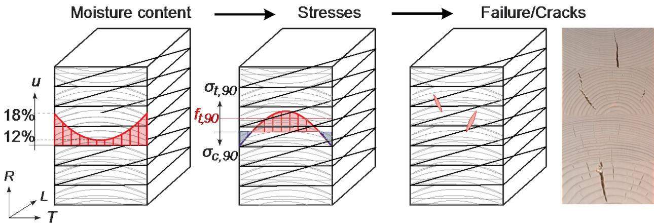
Figure 1: Moisture and stress distribution as well as failure of the cross section for an adsorption process
