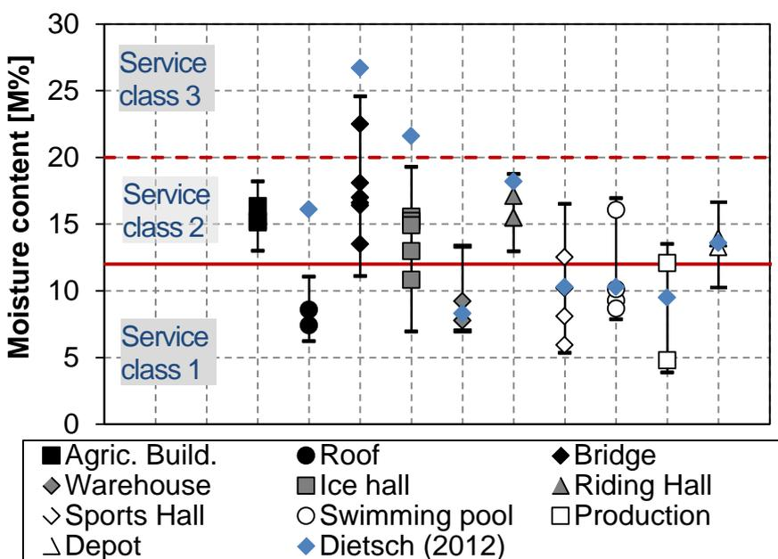
Figure 9: Average moisture content in typical timber building constructions and relation to service classes according EN 1995-1-1:2004
