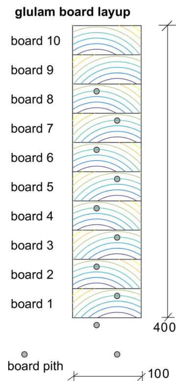
Figure 18: Glulam beam 100/400 mm with alternating pith location on +/- 15 mm from the centerline and 50 mm under board edge
