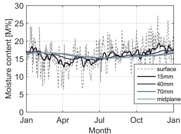
Figure 13: Seasonal moisture content developments on a bridge on a 200 mm wide beam
