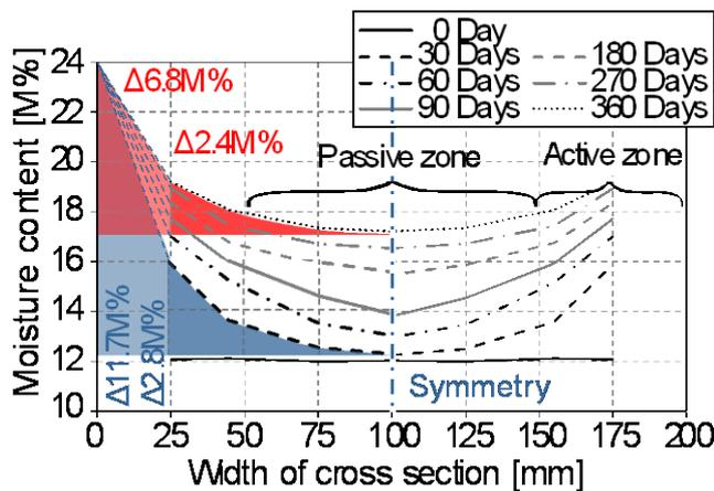
Figure 11: Experimental results of moisture distribution in radial direction for the adsorption process, 200/200/200 mm
