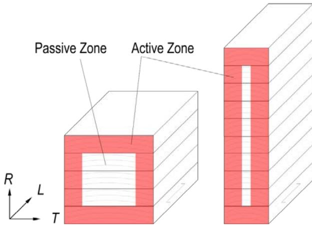
Figure 15: Differentiation of cross section in active and passive zone
