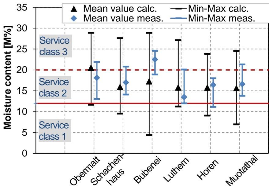
Figure 10: Average moisture content in typical timber building constructions and relation to service classes according EN1995-1-1:2004
