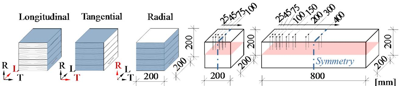
Figure 2: Test specimens with sealed surfaces in blue (top) and position of measuring points for the 200 mm and 800 mm long specimens (bottom)
