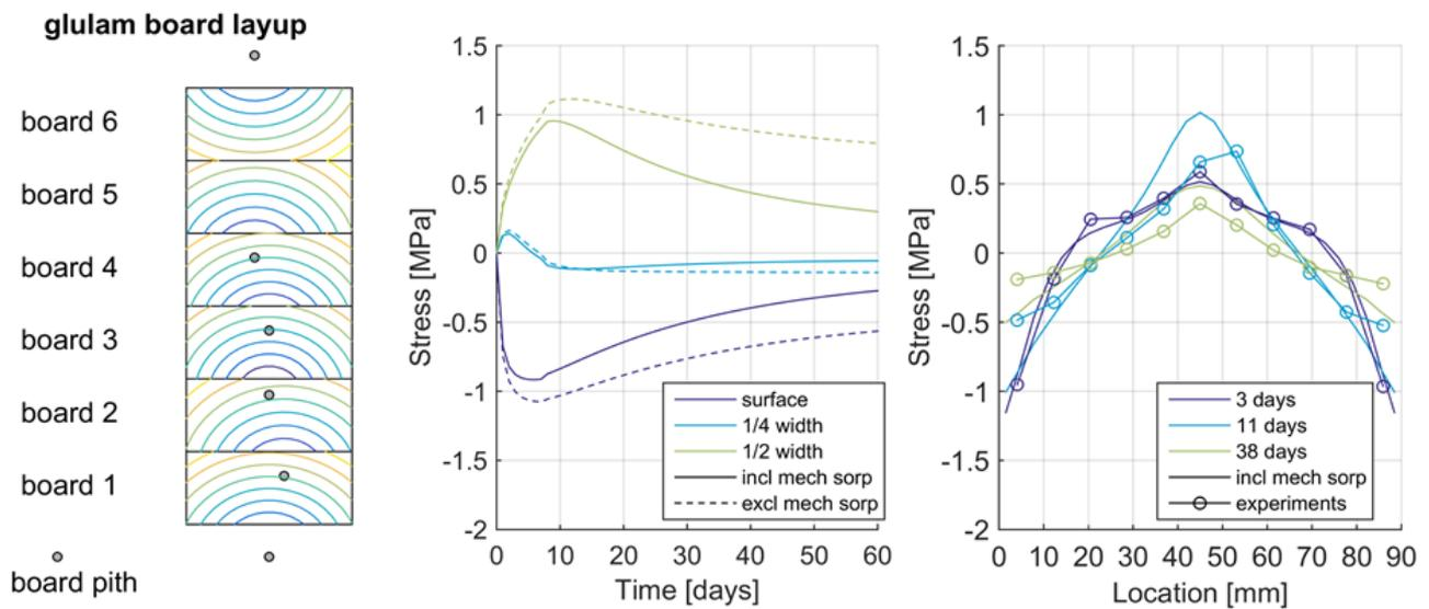
Figure 16: Development of moisture induced stresses in- or excluding time dependent effects in a six layered glulam beam tested in Jönsson (2004).
