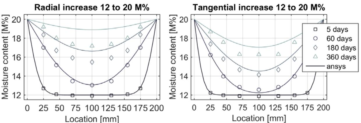
Figure 8: Comparison of experiments and simulations of wetting process in radial and tangential direction of a 200 mm wide beam
