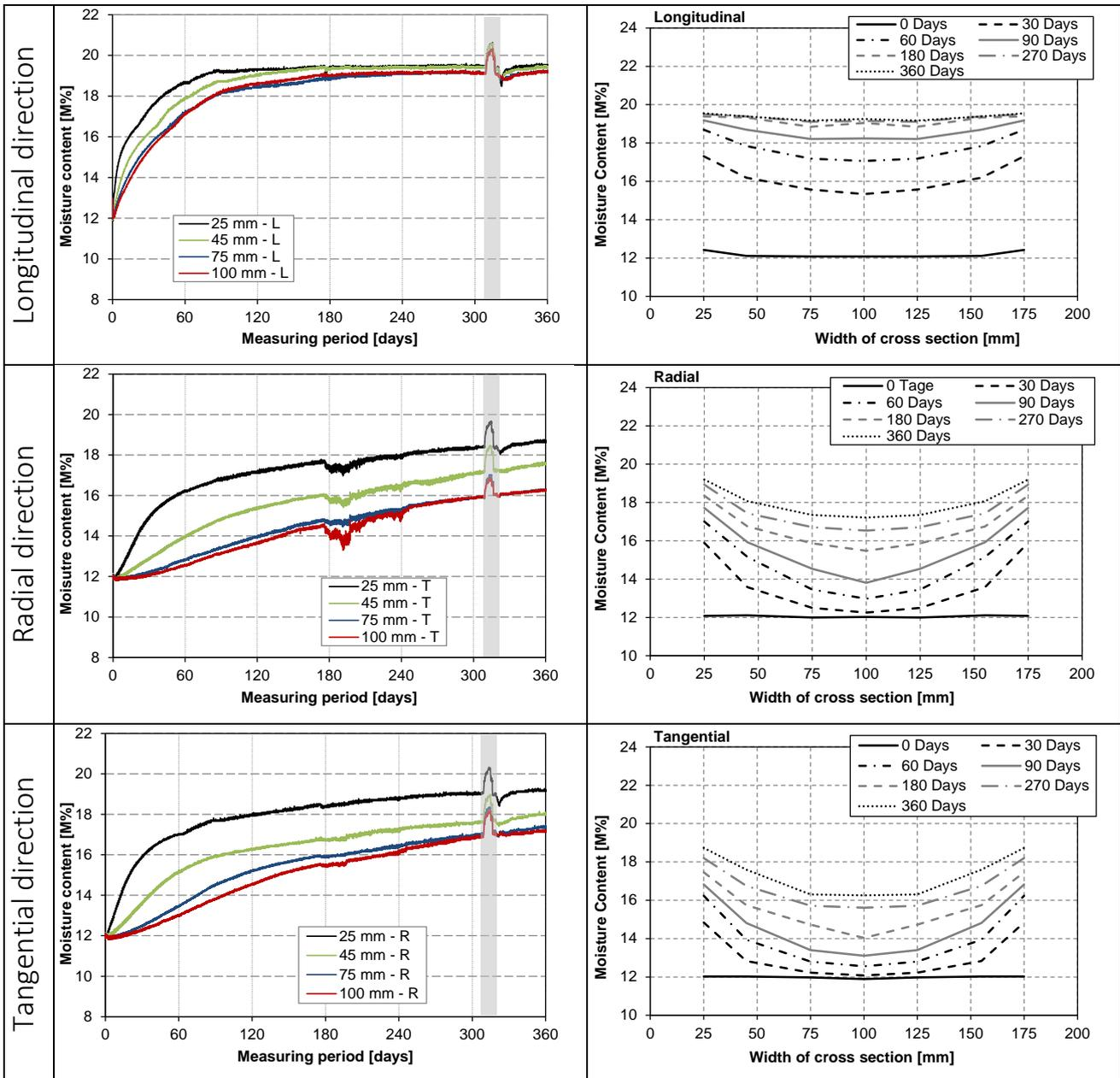
Figure 3: Moisture content development over time and cross section for the three material directions
