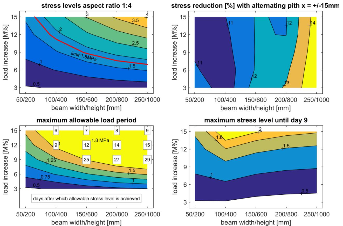
Figure 19: Stress levels, differences of alternating pith locations, maximum allowable loading time, and tension stress levels after 9 days
