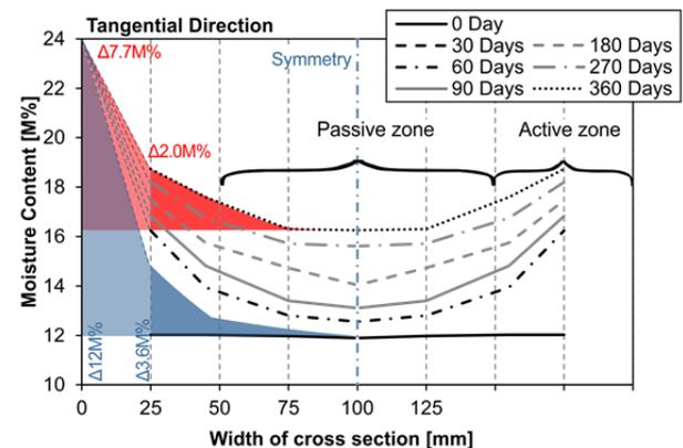
Figure 15: Experimental results of moisture distribution in tangential direction for the adsorption process, 200/200/200 mm
