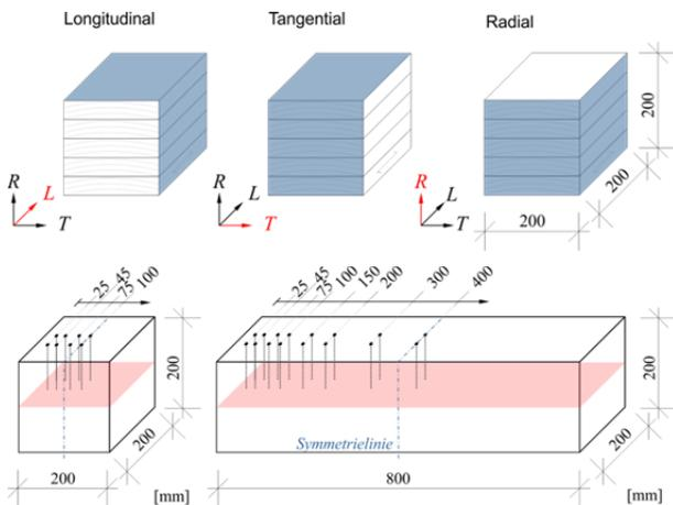
**Figure 2:** Test specimens with sealed surfaces in blue (top) and position of measuring points for the 200 mm and 800 mm long specimens (bottom)
