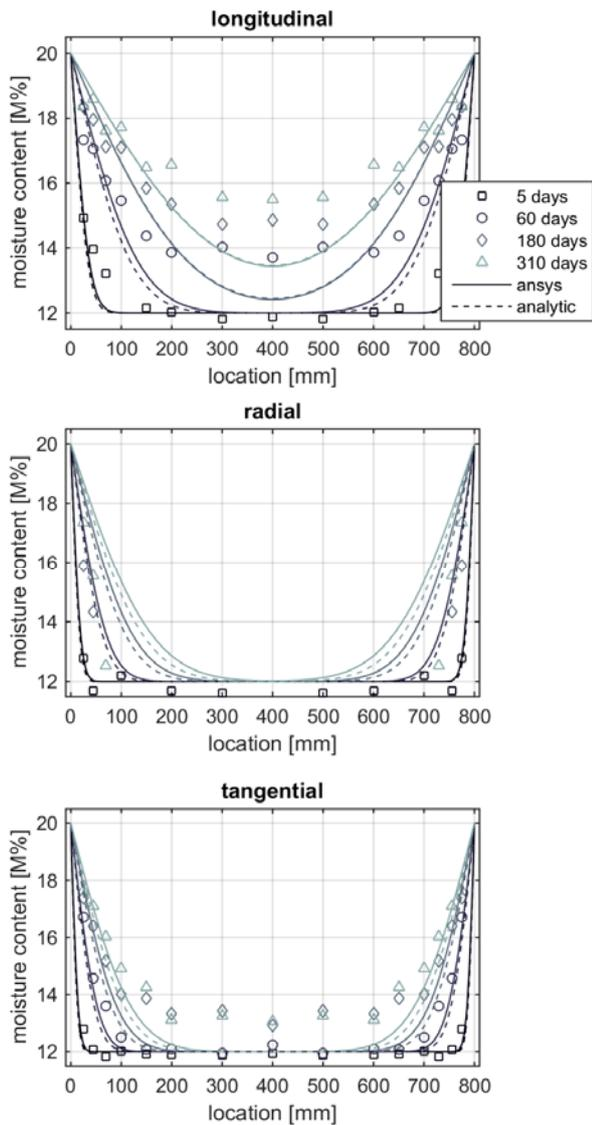
**Figure 10:** Comparison of laboratory experiments with simulations and analytical equations on 800 mm wide specimens.
