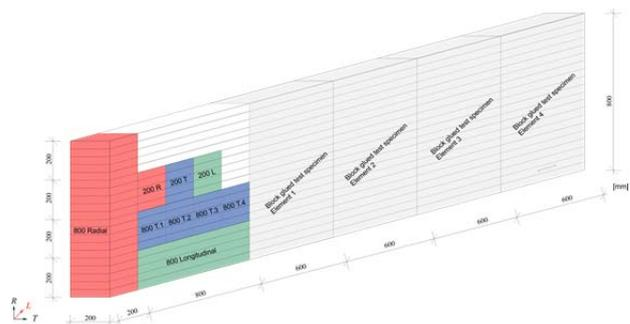
Figure 1: Cutting plan of glued laminated timber member
