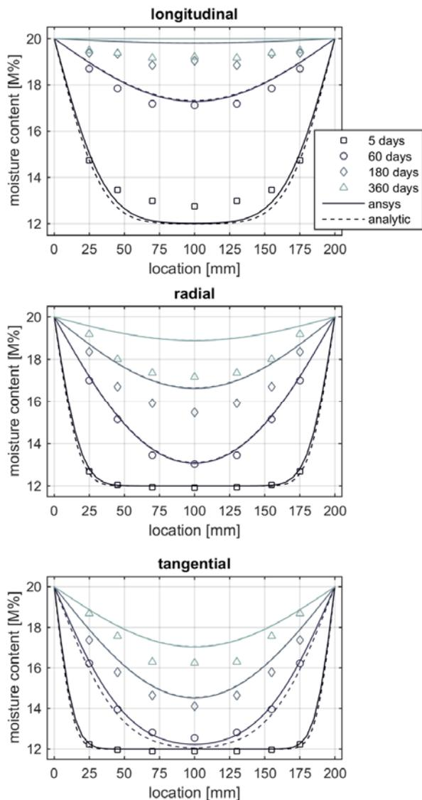
**Figure 9:** Comparison of laboratory experiments with simulations and analytical equations on 200 mm wide specimens
