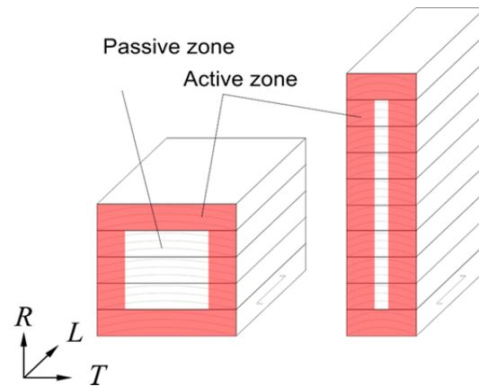
Figure 14: Differentiation of cross section in active and passive zone
