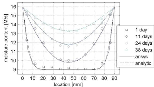
**Figure 8:** Comparison of experiments with numerical simulations and analytical equations on 90 mm wide specimens
