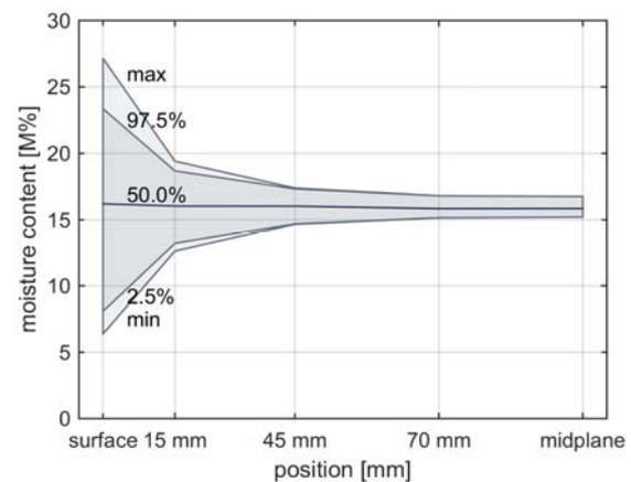
**Figure 12:** Minimum, maximum and percentiles of moisture content calculated for a 200 mm wide beam
