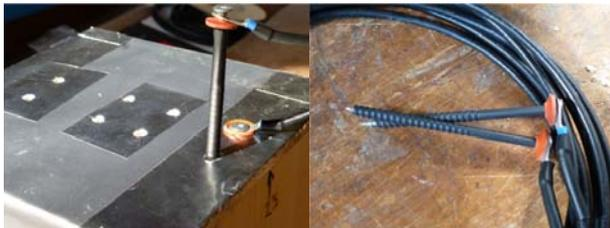
**Figure 3:** Moisture content measuring sensor, insulated stainless steel screws
