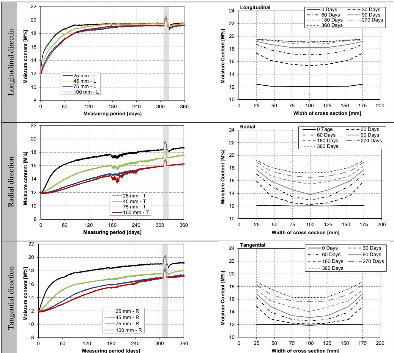
Figure 6: Moisture content development over time and cross section for the three material directions
