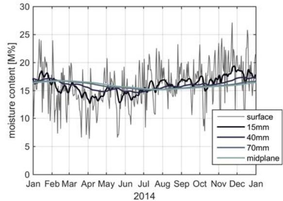
**Figure 11:** Moisture content time traces at different depths of the beams surface throughout 2014
