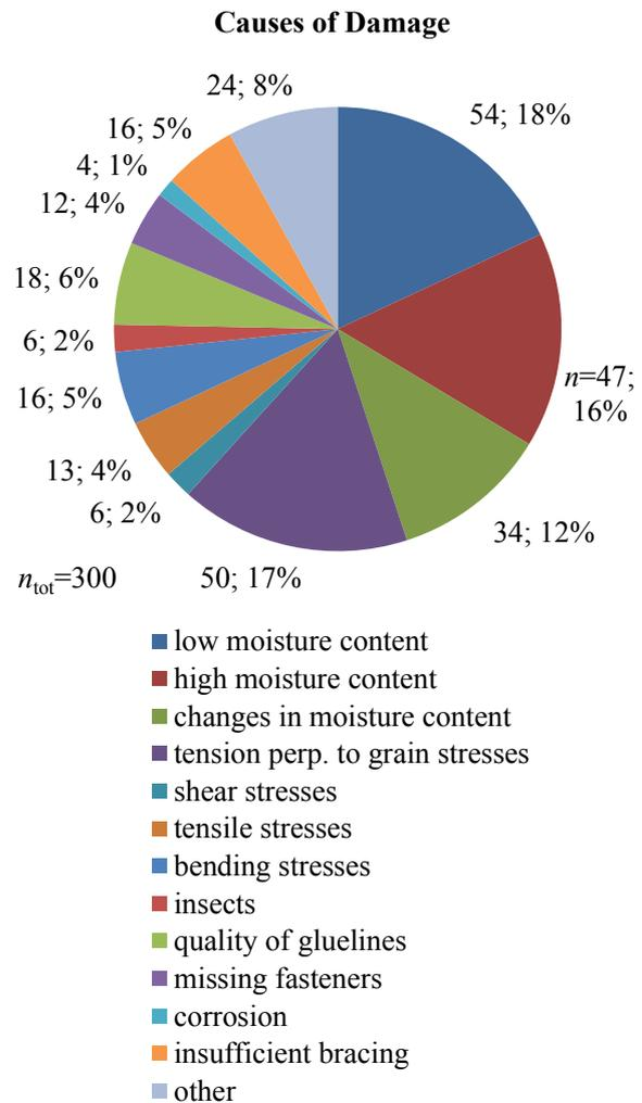
Figure 2: Type of damage from an evaluation of 245 assessments of large-span timber structures [5]
