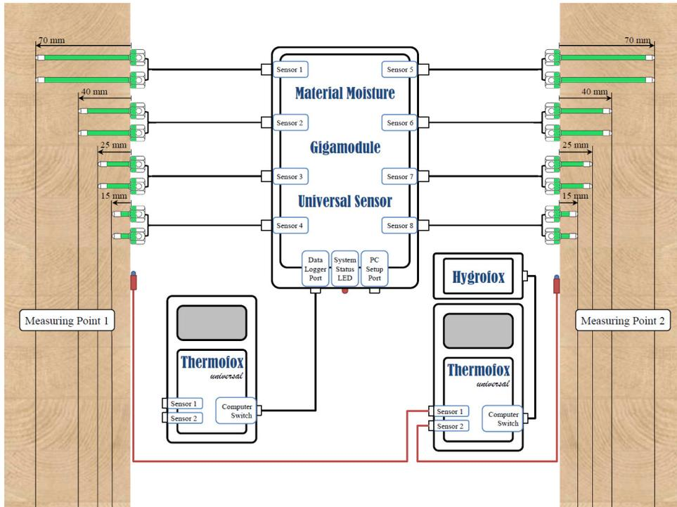
Figure 7: Systematic presentation of the measuring equipment
