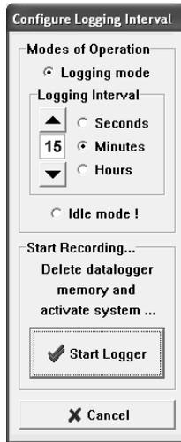
Figure 9: Setting the Thermofox Maxi's measuring interval
