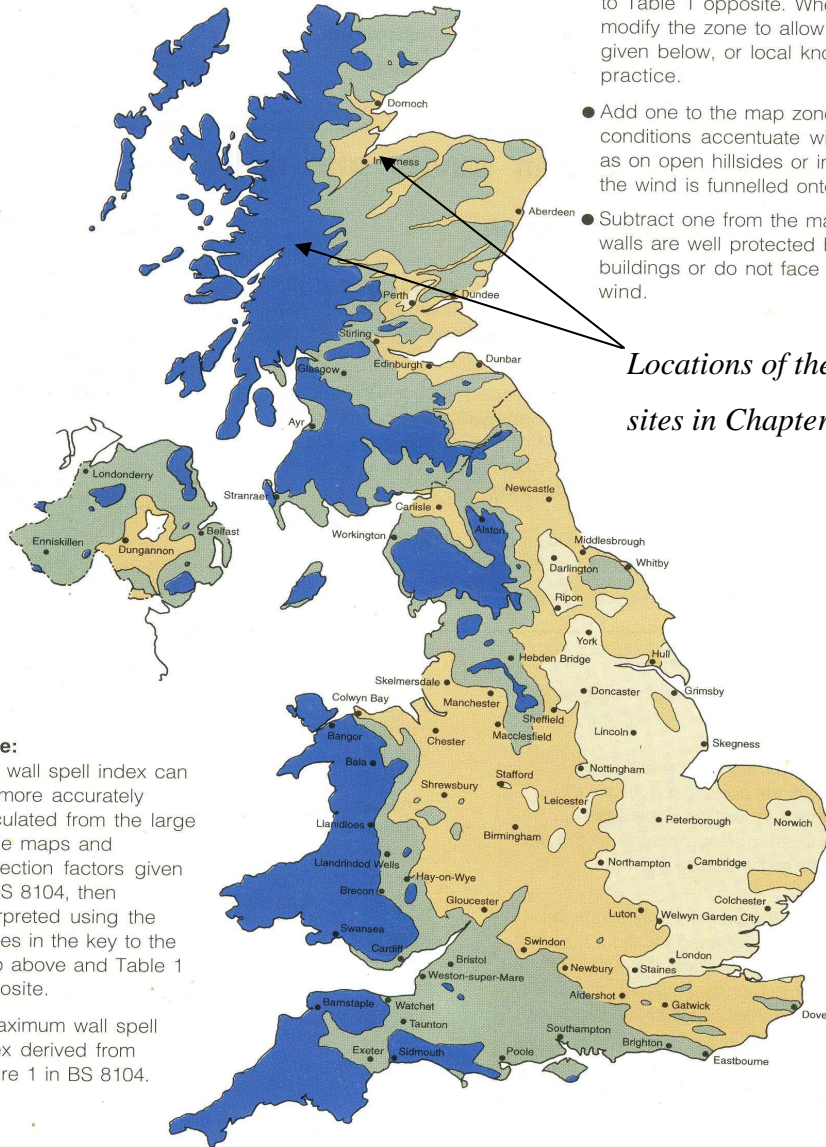
Figure 2.6 WDR exposure zones for masonry walls in BR 262 (map courtesy of BRE [11])
