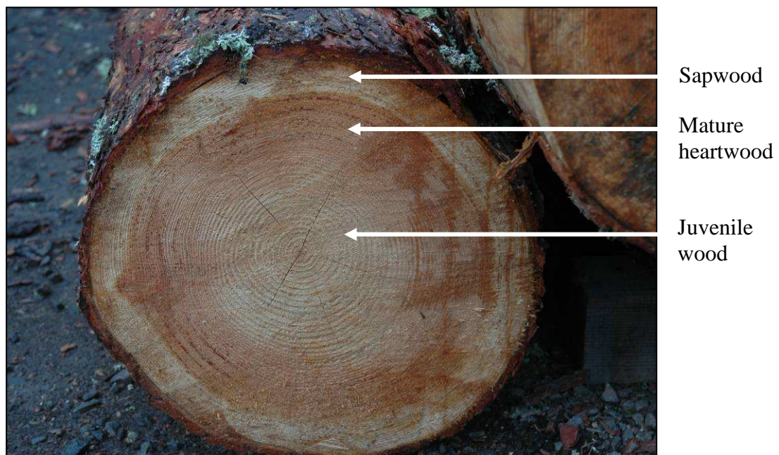
Figure 5.1 A butt log of European larch showing a change in colour and working properties at around the 15 th growth ring
