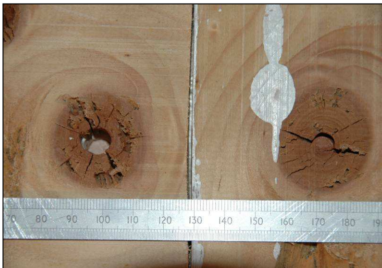
Figure 6.16 Two intergrown knots showing how the centre breaks and can become detached.
