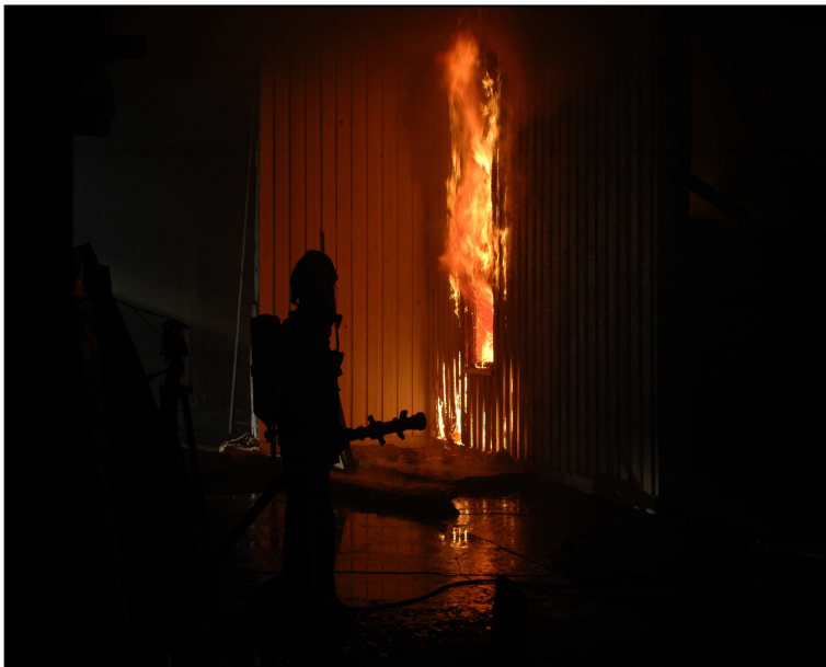
Figure 7.7 View of the facade 53 minutes into the test. The cladding has burnt through above the window and on each side of the horizontal cavity barrier at first floor level. The cavity linings are alight at ground level.
