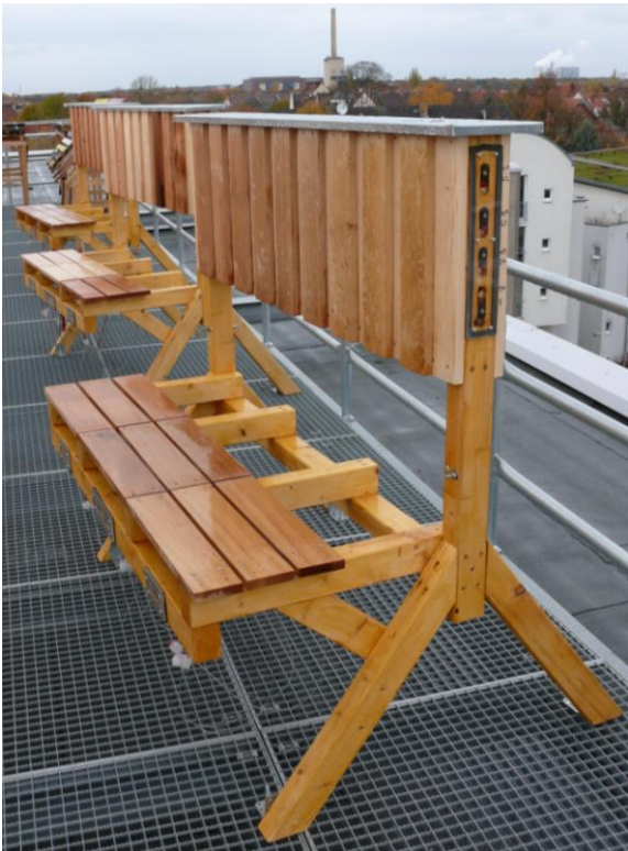
Figure 1: Combined facade and decking elements made from different wood species
