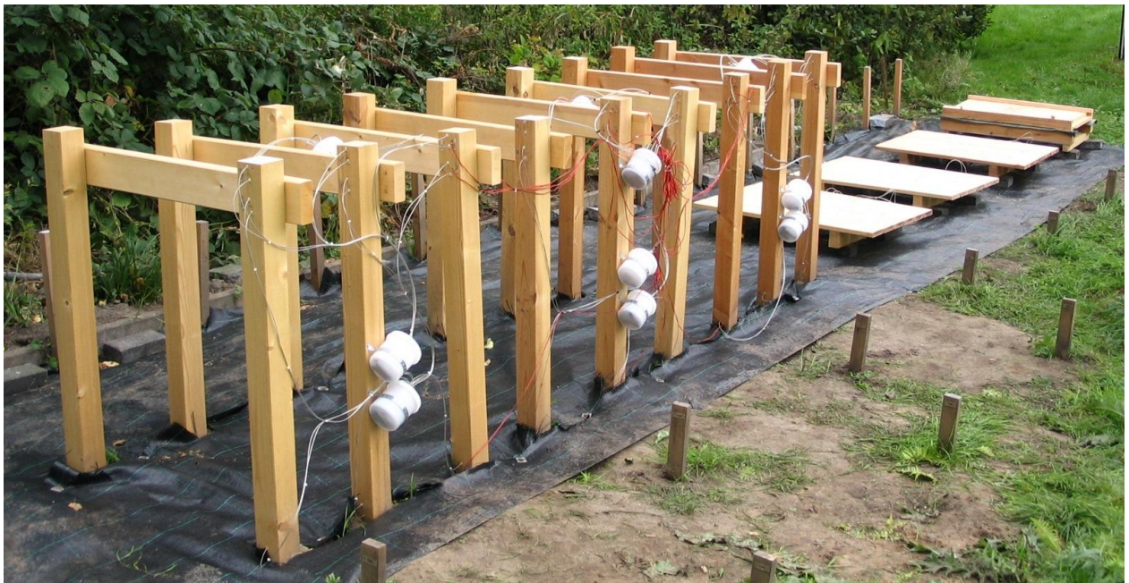
Figure 4: Instrumented fence and decking elements protected from grass growth by a horticultural foil
