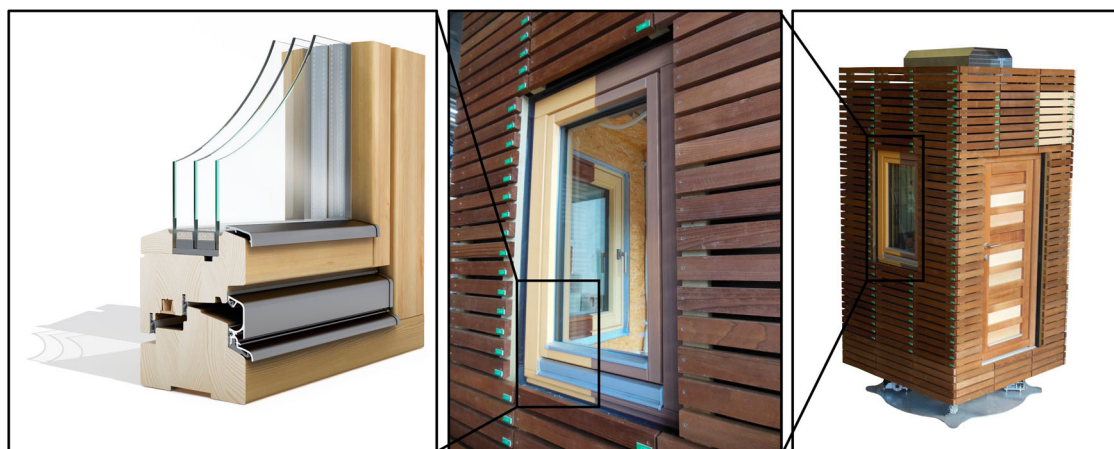
Figure 1. Test cube (right), detail of installed window and facade elements (middle) and detail of window profile (left).
