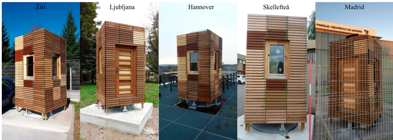
Figure 2. Test cubes with installed test windows and facade elements at different locations.
