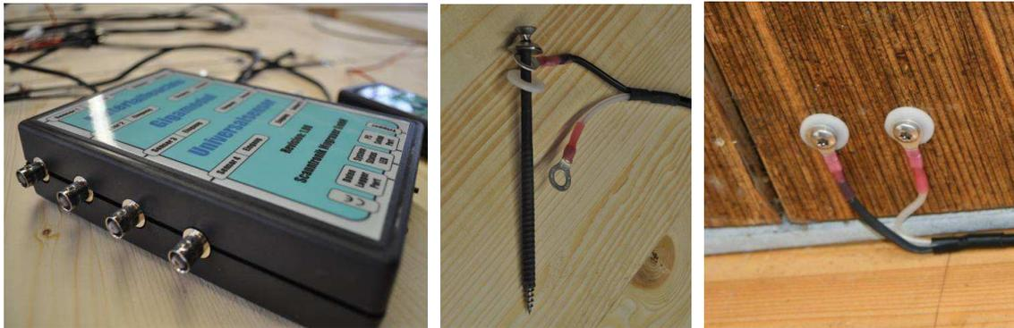
Figure 2. Measurement equipment: Gigamodul© (left), electrode (middle) and installed (right)
