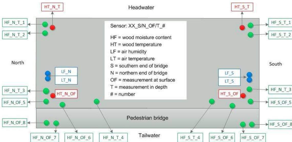
Figure 3. Layout of measuring points including sensor names
