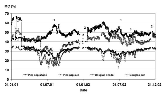
Figure 7.4-4. Courses of moisture content (MC) of pine sapwood and Douglas fir heartwood specimens, sun-exposed and shade-exposed in double-layer test sets in Stuttgart; days with a minimum air temperature below  $0^{\circ}$ C were not considered (Marks 1 to 3 indicate characteristics of the moisture course explained in the text).
