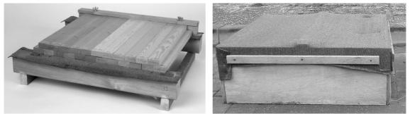
Figure 7.4-1. Left: Photograph showing the double-layer set-up with the upper layer shifted 25 mm horizontally to the lower layer. Specimens are separated with bitumen foil from CCB-impregnated support beams. Right: Artificial shading by textile sheet of double layer test set.
