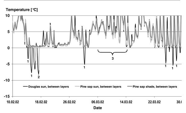
Figure 7.4-6. Course of temperature between pine sapwood layers (sun-exposed: light grey line; shade-exposed: dark grey line), and sun-exposed Douglas fir layers (black line) of double-layer test sets in Hamburg in spring 2002 (Marks 1 to 3 indicate characteristics of the temperature course explained in the text).
