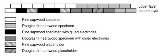
Figure 7.4-2. Scheme of double layer test set up and distribution of specimens containing electrodes for MC measurements.
