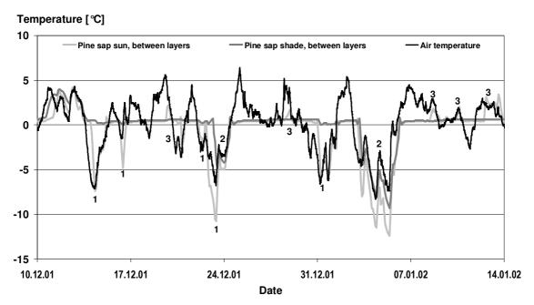
Figure 7.4-5. Course of temperature between pine sapwood layers (sun-exposed: light grey line; shade-exposed: dark grey line) of double-layer test sets and corresponding air temperature (black line) in Hamburg in winter 2001 (Marks 1 to 3 indicate characteristics of the temperature course explained in the text).
