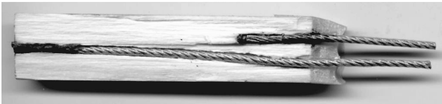
Figure 7.3-4. Longitudinal cut through a substitute dowel made from Scots pine sapwood, impregnated with tebuconazole in white spirit, containing a pair of glued electrodes.
