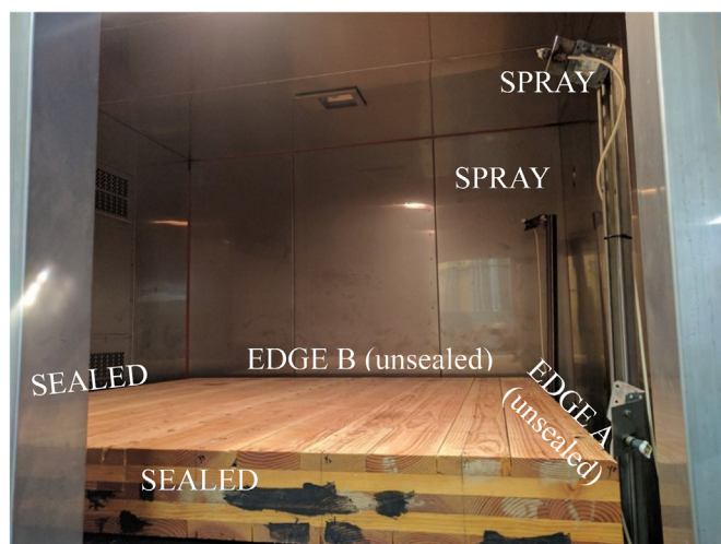
Fig. 1. The DF CLT panel installed in the environmental chamber.
