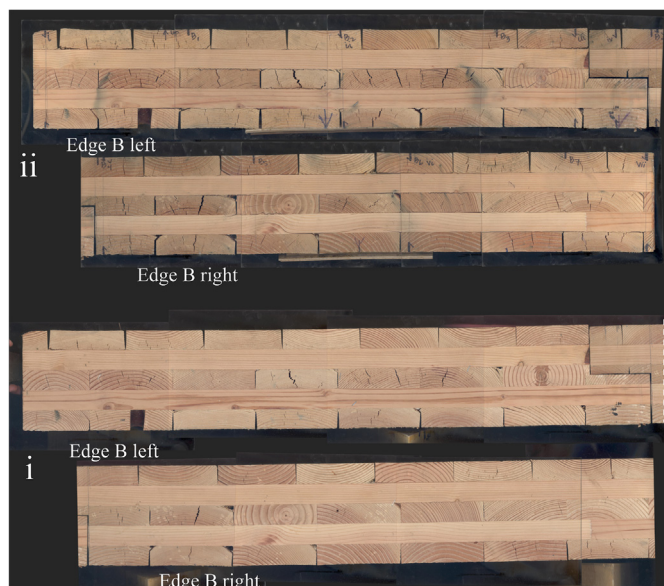
Fig. 14. Edge B before and after weathering. (ii): Edge B after two cycles of weathering. (i): edge B before weathering.
