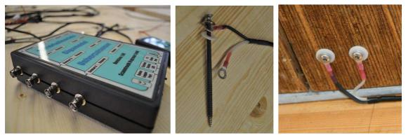
Figure 2. Measurement equipment: Gigamodul© (left), electrode (middle) and installed (right)
