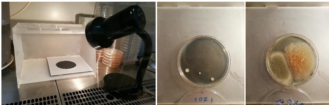
Figure 23: PhotoBox (left) and resulting pictures of PC-agar (middle) and ME- agar plates (right)
