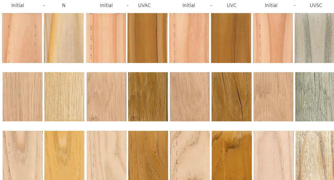
Figure 61: Scans of Douglas (upper row), oak (middle row) and chestnut (third row), exposed to NSWE for 6 weeks
